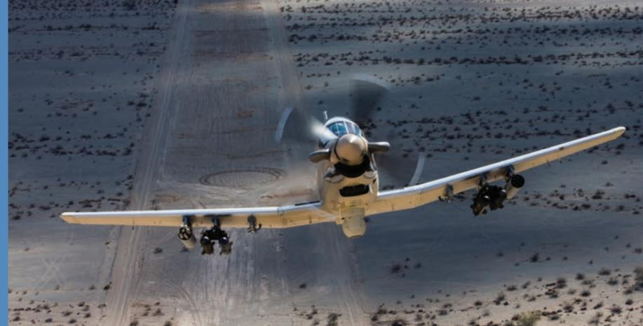
**Above:** The AT-6 demonstrated a max-weight take-off and landing distance of less than 5,000ft in the hot and high altitude conditions of Holloman AFB. **Beechcraft/ Paul Bowen**
